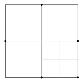
If your survey requires that you bound the section, you are required at a minimum to file Certified Corner Records for the four quarter section corners. If the survey is for the purpose of locating, for example, the SE1/4 of the section, then you would also file a Certified Corner Record for the SE corner of the section as well as for the four quarter section corners.
