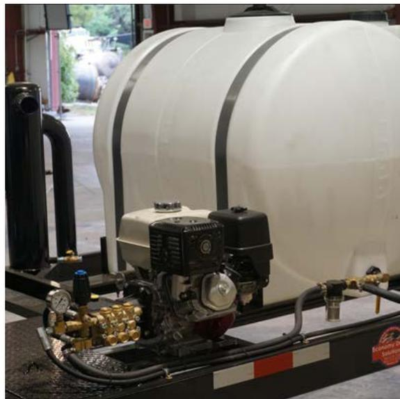
The Lo-K-Tor consists of a pressure pump, water tank and wand, trailer and vacuum pump and debris tank for a base price of about \$36,000 each. The previous owner was selling about one unit per month.
