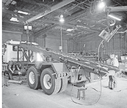
Roll-off hoists are installed for use with waste containers at Texoma Mfg. (PHOTO PROVIDED)
