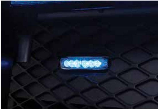
MicroPulse® C Series lights come with an optional stud mount that provides easy installation in the pre-drilled grille of the Ford Police Interceptor Utility.
