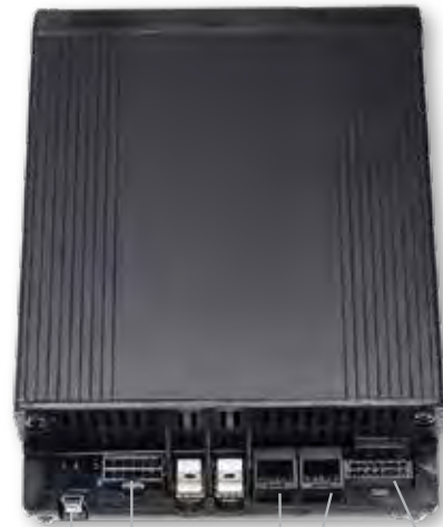
USB 12 Relay Outputs (7) programmable input circuits, speakers and radio input Convergence Network ports
