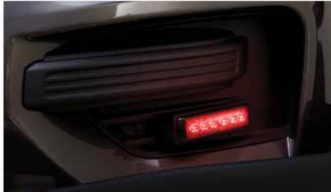
MicroPulse Ultra light heads can be programmed to operate as a single unit or in synchronization with multiple MicroPulse light heads.
