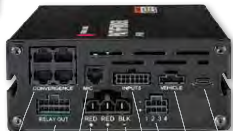
Convergence Network ports RELAY OUT MIC RED RED BLK INPUTS 1 2 3 4 VEHICLE OBDII USB-C Siren power Ground Speaker outputs (16) programmable relay outputs Remote microphone (7) programmable input circuits and radio input
