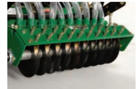
The curved shape of the discs direct the seed into the soil slits for ultimate seed-to-soil contact and maximum germination.
