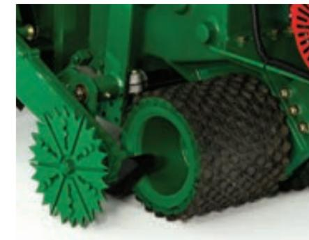
A forward metering wheel measures accurate sod cut lengths.
