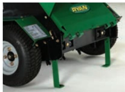
Built-in jack stands help to provide easy maintenance, including chain lubrication, tine replacement, and changing rear tires.
