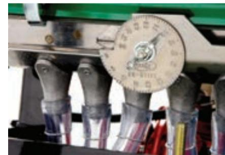
The seed rate control allows for seeding at variable rates and for different grass varieties and applications.
