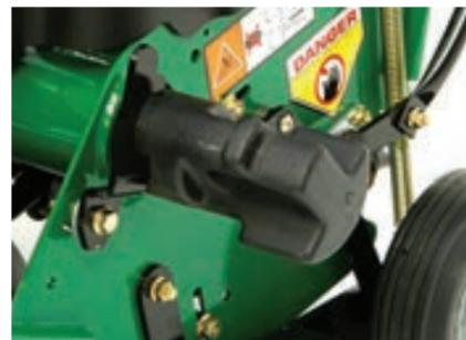
Weights are easily and conveniently removable for easier lifting and quicker, less strenuous transportation.
