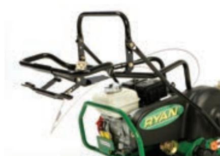
The fold-down handle allows the machine to take up less space during transport or storage. (Lawnaire IV only)
