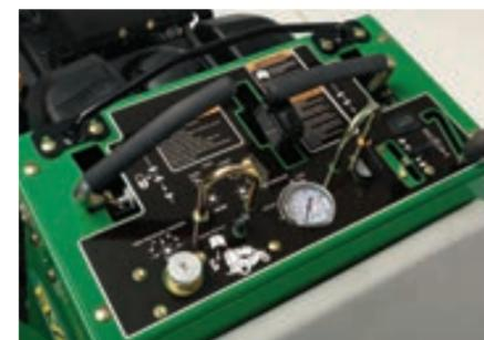
The intuitive control panel features a hydraulic pressure gauge with easy-to-read dial for management of down pressure under various soil conditions.
