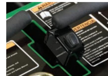
Tine lift switch to raise and lower tines conveniently located near control lever.
