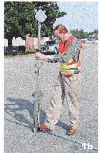
2. Lift the stand with the Vertical Upright so that the Legs lock in the first Locking Hole. When setting up for uneven terrain the Legs may be adjusted to different holes as needed by tilting the stand to relieve the pressure on the Locking Pins and then releasing and repositioning them. There are two additional leg positions available.
