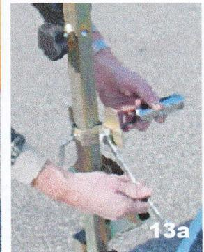
13. To display a rectangular Supplemental Sign under the Primary Sign, use one of the optional supplemental Roll-up Sign Mounting Brackets (Figure 13a) to capture the ribs on a roll-up and use the anti-rotation Velcro strips to help secure the sign (Figure 13b). For a rigid sign use the standard Roll-up Sign Mounting Bracket in the inverted orientation (Figure 13c) to capture the top of the sign with the bottom of the sign held by the bottom Rigid Sign Holder (Figure 13d).
