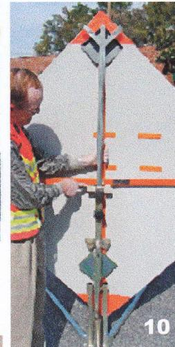
10. To mount a roll-up sign at the 60" height, leave the Roll-up Sign Mounting Bracket loose and place the Horizontal Rib behind and the Vertical Rib between the Ears of the Roll-up Sign Mounting Bracket.
