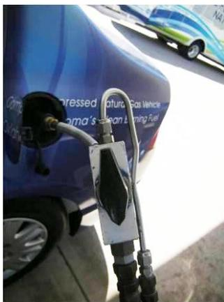
2.5.3. Pull the external cover (rubber) back toward you and pull the nozzle to the quick-connect fitting off the vehicle.
