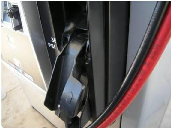
2.5.2. Turn lever on valve off. The pointed end of the valve should point away from the dispenser-end of the hose nozzle.
