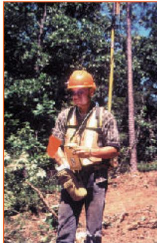
*Survey crews use global positioning systems (GPS) to ensure accuracy of placement of source and receiver lines.*
