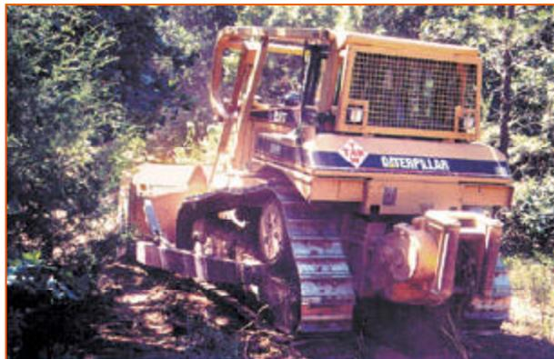
*In timbered areas, a path may need to be cleared for the source lines. Paths for receiver lines are usually cleared by hand and need be only about four feet wide.*
