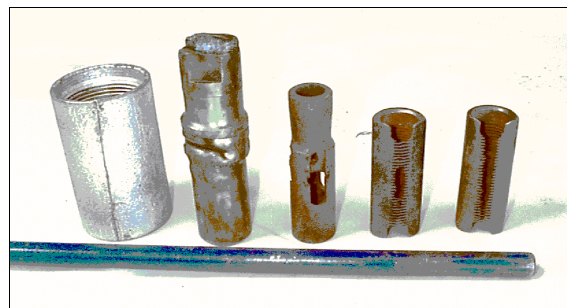
Figure 3. A split collar, damaged brass pump part, corrosion damage, and two worn sucker rod boxes.
