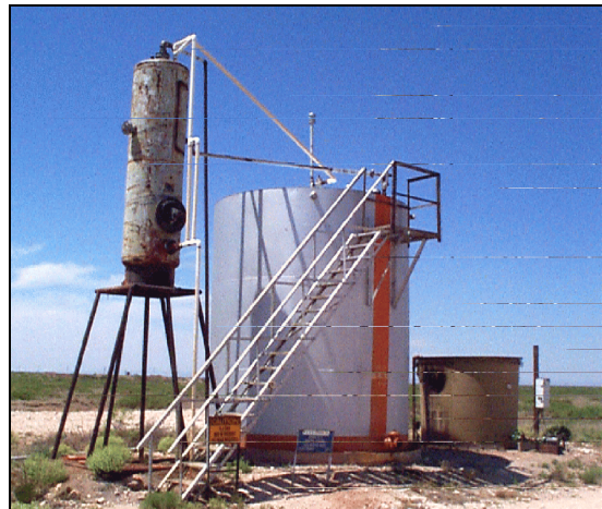
Figure 5. Atmospheric gun barrel made from a vertical separator and a pipe platform.
