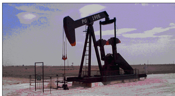
Figure 1. A conventional beam-style pumping unit.
