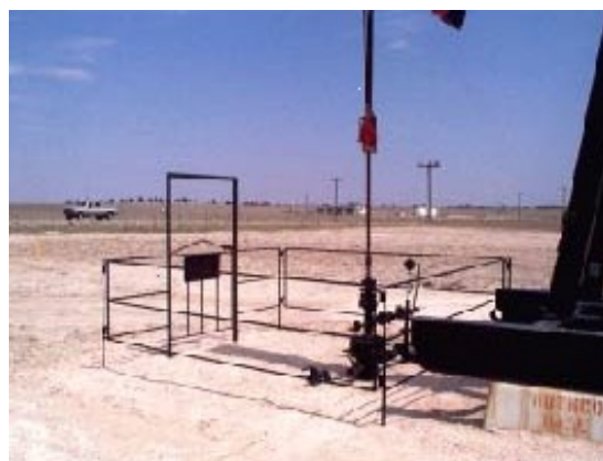
Figure 2. Fences may have to be installed around equipment to keep livestock out.
